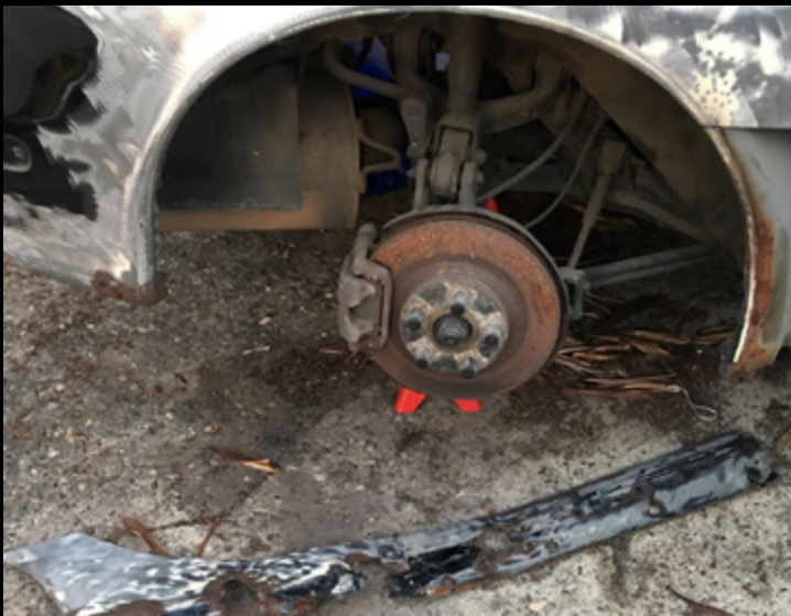
Hidden rust beneath the pre-installed body kit
